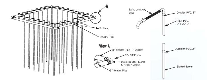
The wellpoint system is used to lower the water table to allow construction of buildings and civil works. All pipes shown bring water from the ground to the suction port in the pump. Discharge from the pump is then either directed to a canal or catch basin depending on site conditions.
