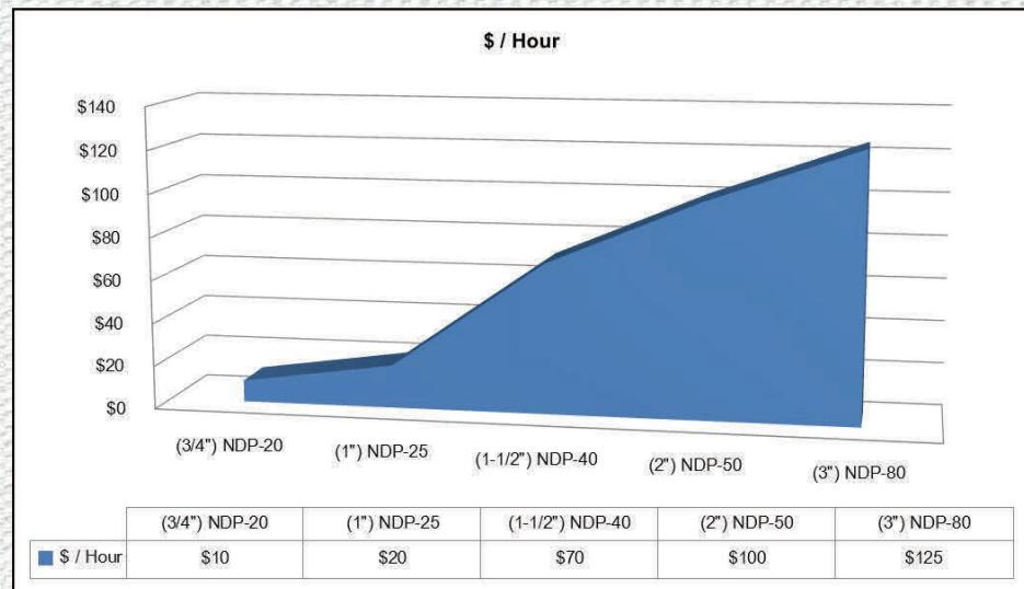
Savings are based on 7.5¢ / per Kilowatt Hour, running dry at 100 PSI.
