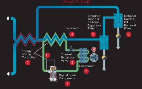
While the compressor continues to run, the Energy Saving Controller (7) automatically energizes and de-energizes the solenoid valve (8) to load and unload the compressor. This precisely controls the flow of the refrigeration circuit to exactly match your load conditions. We maintain a stable 38° F pressure dew point, and provide you with maximum energy savings.
