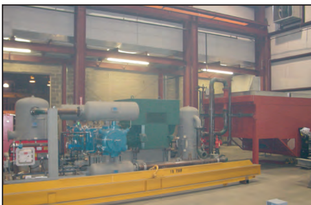
■ (Left) A 700 hp (522 kW), 900 rpm single-stage compressor package is shown in Dearing Compressor and Pump Co.'s new high-bay fabrication addition. The package includes an Ariel JGH/2 driven by a Reliance electric motor and a separate R&R Engineering cooler. It will be used for a gas processing plant in Virginia for nitrogen removal. (Right) Two Dearing Compressor & Pump Co. three-stage gas gathering and boosting compressor packages are shown being installed at a customer site near Clarksburg, West Virginia, U.S.A. Each package includes a Caterpillar G3516 gas engine driving an Ariel JGE/4 compressor at a rated speed of 1400 rpm.
