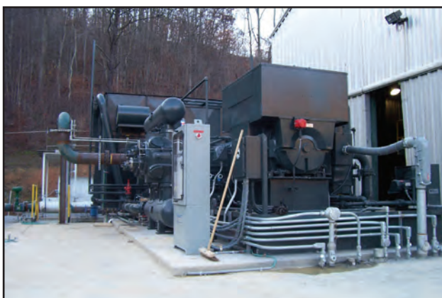
■ (Above) A Dearing three-stage 1250 hp (932 kW) electric motor-driven Ariel JGK/4 compressor package shown in an Appalachian Basin gas gathering application. (Below) Dearing Compressor & Pump Co. package designs are engineered using AutoCAD Inventor 3-D modeling software. Shown here is a two-stage Caterpillar G3516 engine with an Ariel JGE/4 compressor.
