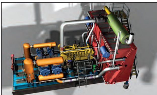
■ (Above) A Dearing three-stage 1250 hp (932 kW) electric motor-driven Ariel JGK/4 compressor package shown in an Appalachian Basin gas gathering application. (Below) Dearing Compressor & Pump Co. package designs are engineered using AutoCAD Inventor 3-D modeling software. Shown here is a two-stage Caterpillar G3516 engine with an Ariel JGE/4 compressor.
