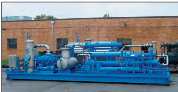
■ This Dearing package is ready for service in a New Jersey, U.S.A., wastewater treatment plant, compressing digester gas for use as gas turbine fuel. In addition to an electric motor-driven rotary screw compressor, the system includes a built-in chiller to remove water.
