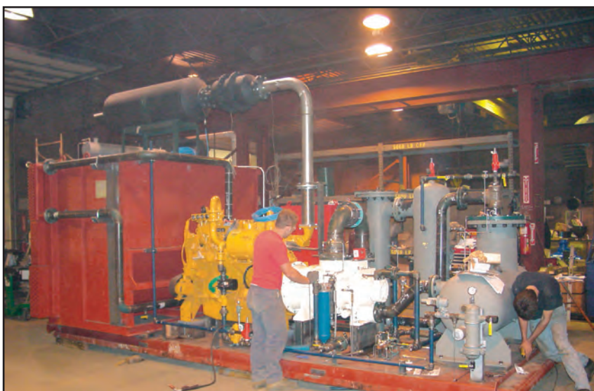
■ This Caterpillar G3406NA driven Gardner Denver SSQG rotary screw compressor is being fabricated in Dearing Compressor and Pump Co.'s shop in Youngstown, Ohio, U.S.A. Destined for a wellhead compression application in Western Pennsylvania, it is rated at 215 hp (160 kW) at 1800 rpm.
