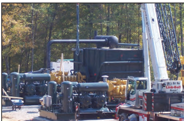
■ (Left) A 700 hp (522 kW), 900 rpm single-stage compressor package is shown in Dearing Compressor and Pump Co.'s new high-bay fabrication addition. The package includes an Ariel JGH/2 driven by a Reliance electric motor and a separate R&R Engineering cooler. It will be used for a gas processing plant in Virginia for nitrogen removal. (Right) Two Dearing Compressor & Pump Co. three-stage gas gathering and boosting compressor packages are shown being installed at a customer site near Clarksburg, West Virginia, U.S.A. Each package includes a Caterpillar G3516 gas engine driving an Ariel JGE/4 compressor at a rated speed of 1400 rpm.
