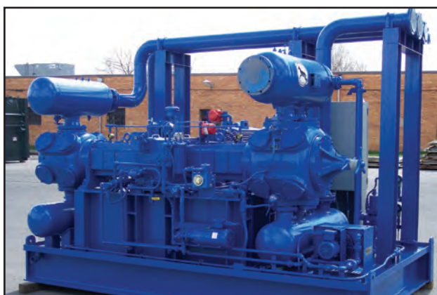
■ This recently completed 125 hp (93 kW) motor-driven two-stage nonlube Ariel JGJ/2 compressor is ready for shipment from Dearing Compressor and Pump Co.'s Youngstown, Ohio, U.S.A., plant for service in an LNG gas boil-off application.
