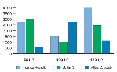
Calculations (using published data) are based on the cost of providing the volume of air that Gardner Denver Electra-Saver II compressors can deliver in 8000 hours (approximately 1 year) of operation at full load. Assumes motor efficiency=.90, cost per kilowatt-hour=\$0.07.
